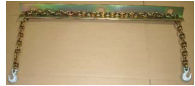
Breaker lift yoke
